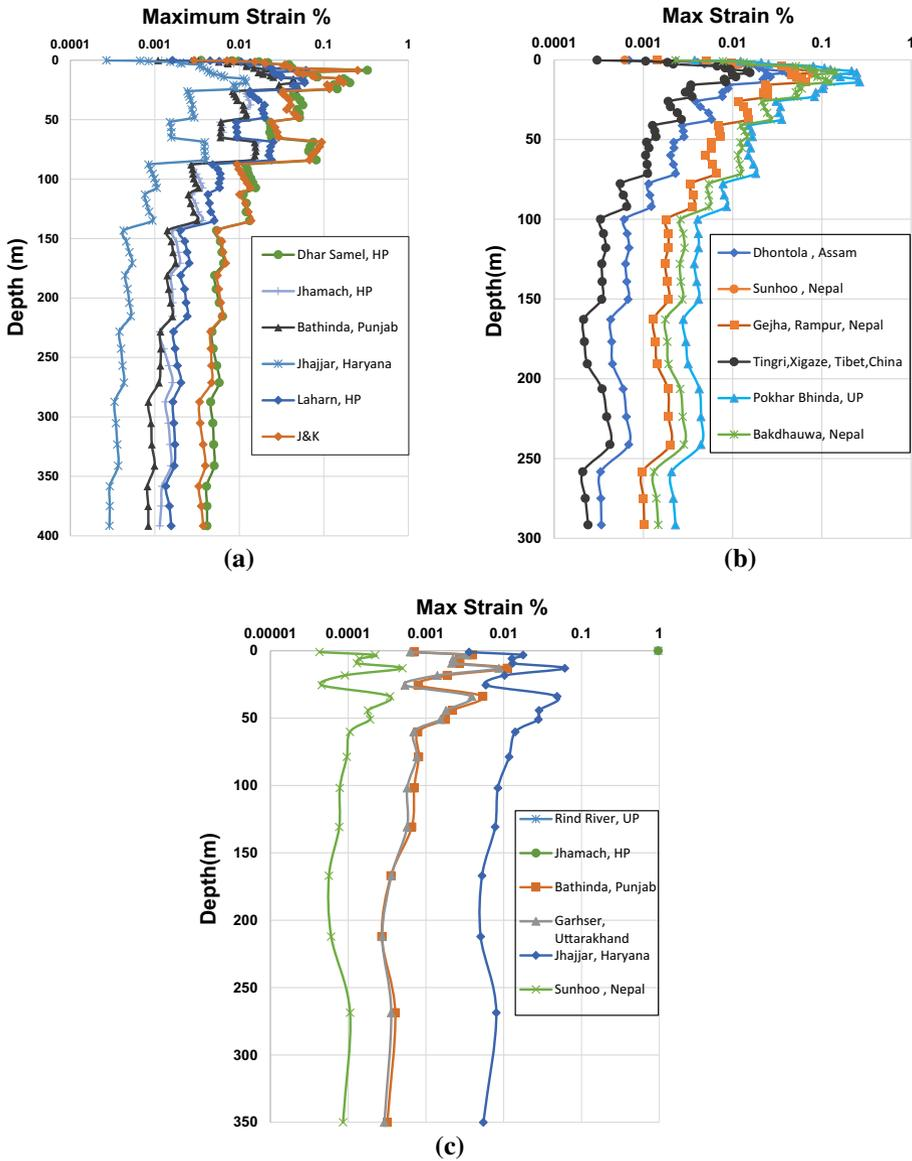
**Fig. 18** Depth-wise variation in maximum strain at a typical site at **a** Punjab Haryana (PHR), **b** Bihar and **c** Uttar Pradesh (UP)
